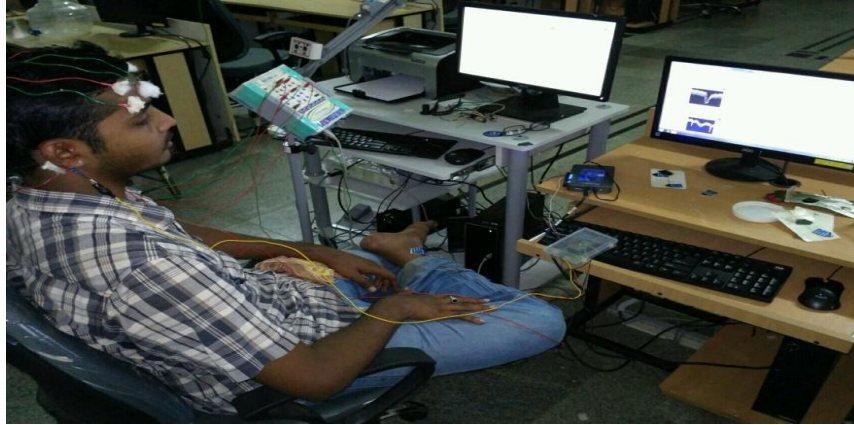
Fig 3.9. Interface of EOG Detector using NI myRIO to Neuromax
